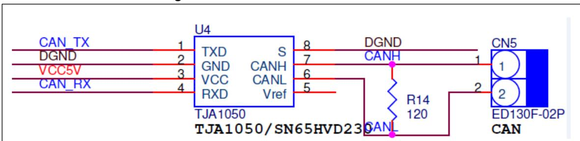
TJA1050 (driver IC) is connected to MCU and CAN bus analyzer. It is mainly used for data conversion.
