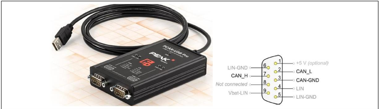
Note: Besides connecting to CAN1\_L and CAN1\_H, the CAN bus analysis device must share the same ground with MCU.
